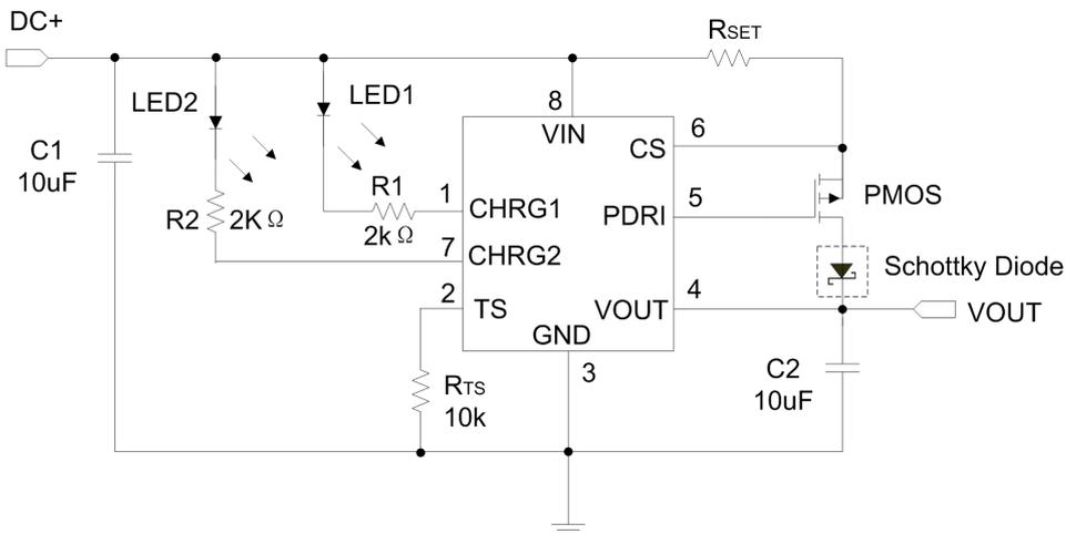
Figure 1: Typical Application Circuit with Two LEDs
